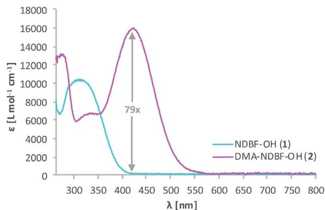
Fig. 2 Comparison of the 1P-absorption spectra of NDBF-OH (**1**, cyan) and its dimethylamino derivative DMA-NDBF-OH (**2**, magenta) in DMSO. The maximum is shifted bathochromically for photocage **2** due to addition of the N(Me)<sub>2</sub> moiety and the absorption at 420 nm is 79 times higher.
