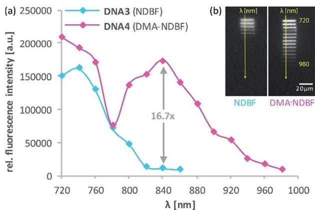
**Fig. 6** (a) 2P-activation of fluorescence (ATTO565) with NDBF and DMA-NDBF, based on (b) intensity measurements in a hydrogel after uncaging at the indicated wavelengths. DMA-NDBF has a red-shifted local maximum at 840 nm.
