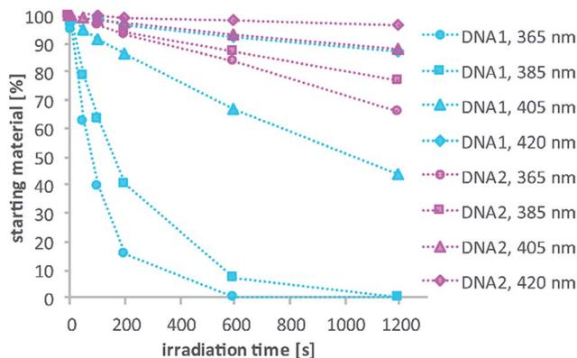
**Fig. 5** Comparison of 1P-photolysis of **DNA1** and **DNA2** at various wavelengths but with the same number of photons per time. Conversion was determined by HPLC analysis. (260 pmol, 13 μl, 0.42 mW in case of 365 nm irradiation).
