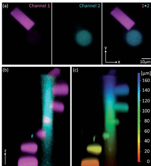
Fig. 8 3D picture of a winding staircase with a one-photon uncaging (420 nm) core and two-photon (840 nm) steps. (a) Channel 1, channel 2 and combination in  $x$ -/ $y$ -plane and (b)  $z$ -/ $y$ -plane. (c) Colour-coded height profile of the  $z$ -/ $y$ -plane (0–160  $\mu\text{m}$ ).
