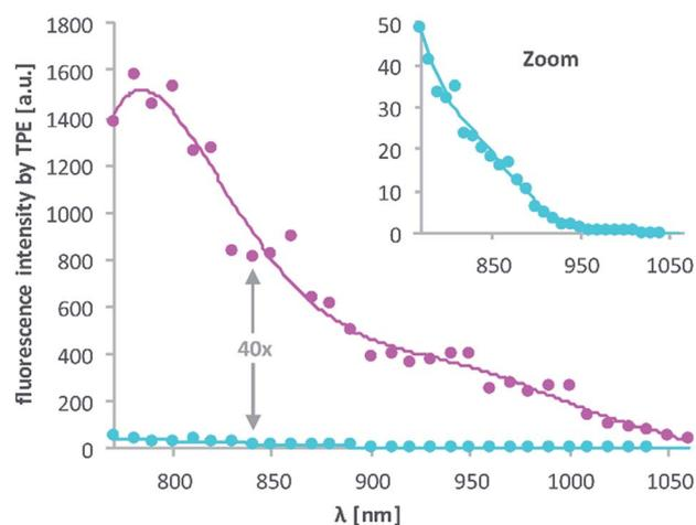
Fig. 3 Excitation spectra resulting from 2PE between 770 and 1060 nm of **1** and **2** in DMSO. The excitation power was set to 1.0 mW and squared dependence tested (ESI<sup>†</sup>). Axes labelling for the "zoom" is the same. Solid lines are averages of the raw data (dots).
