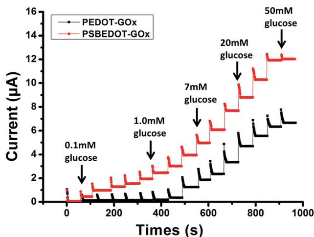
Fig. 2 Amperometric response of the PSBEDOT-GOx (red) and PEDOT-GOx (black) biosensors to the successive addition of glucose in PBS; the concentration of glucose was increased from 0.1 mM to 50 mM.
