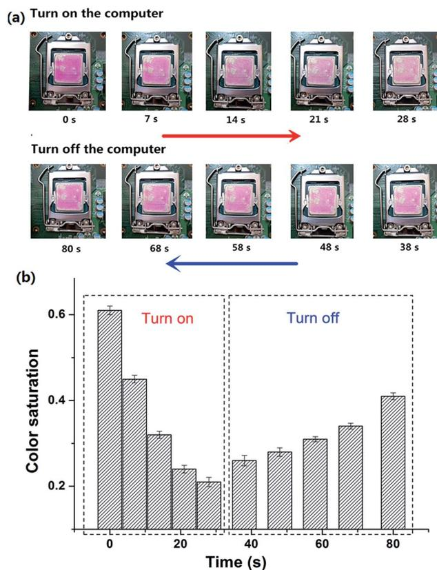
**Fig. 3** (a) Digital images of a **D1-non** coated CPU with different running times illustrating the color changes, and (b) color saturation of the digital images of **D1-non** as a function of the computer running time. The error bars represent standard deviation ( $\pm$ S.D.).
