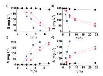
Fig. 4 Aerobic oxidation of DBT (a and b) to DBTO<sub>2</sub> (c and d), plotted as sulfur content, using MUV-2 ( $\blacksquare$ ), MIL-101 (Fe) ( $\bullet$ ), and MIL-100 (Fe) ( $\triangle$ ) and in the absence of a catalyst ( $\bullet$ ) using n-dodecane (a and c) or diesel (b and d). Reaction conditions: 0.012 mmol of Fe catalyst, DBT (1150 mg L<sup>-1</sup>), solvent (10 mL), O<sub>2</sub> (1 atm) and 140 °C.
