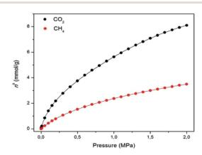
Fig. 3 Gas adsorption isotherms of  $CO_2$  (black) and  $CH_4$  (red) on MUV-2 at 298 K (lines correspond to the best fits). Data at other temperatures are shown in the ESI.†
