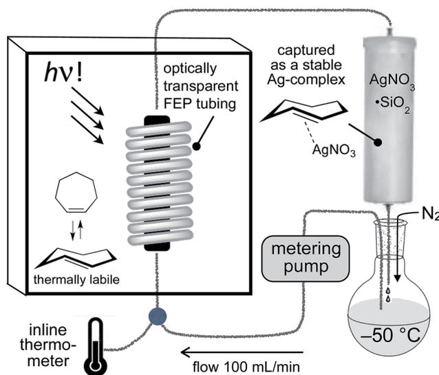
Fig. 1 The apparatus for photoisomerization of carbocyclic *trans*-cycloheptene derivatives was designed to minimize loss of *trans*-cycloheptene due to thermal isomerization by using FEP tubing and inline cooling. For the synthesis of *trans*-1-sila-4-cycloheptenes, photoisomerizations could be carried out at rt using a conventional flow photoisomerization setup.
