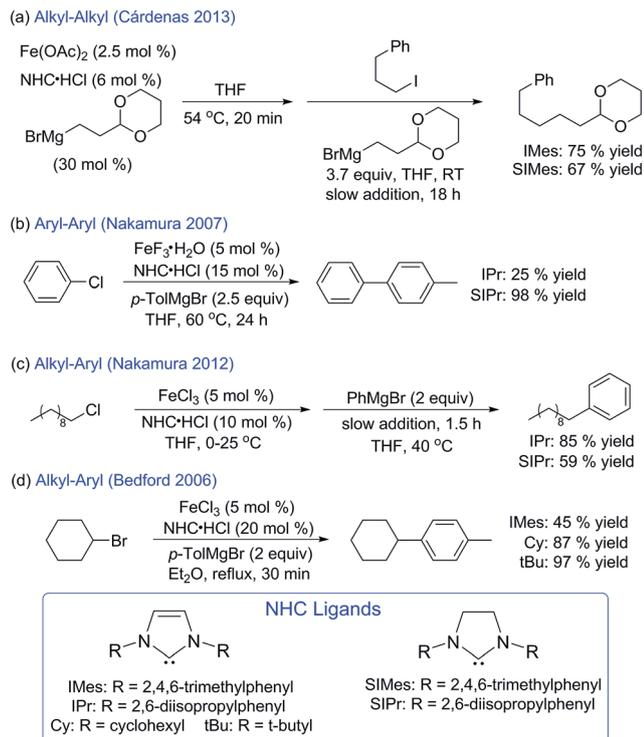
Scheme 1 Examples of iron–NHC catalysed cross-coupling reactions.
