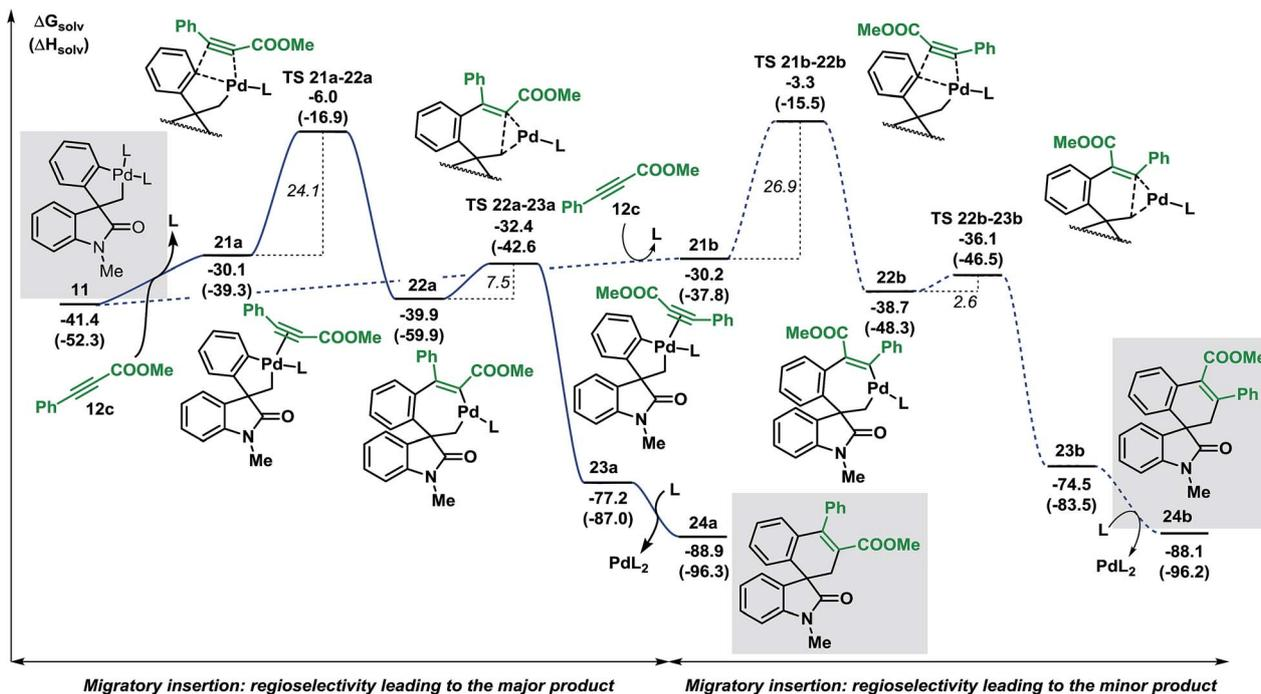
Fig. 7 Computed Gibbs free energy profile explaining the regioselectivity of the migratory insertion of methyl 3-phenylpropiolate **12c** (L = Ph<sub>3</sub>P).
