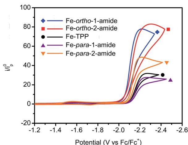
Fig. 3 Cyclic voltammograms of amide-functionalized porphyrins and unfunctionalized Fe-TPP under CO<sub>2</sub> atmosphere. Conditions: 1 mM catalyst, 100 mM phenol, 0.1 M TBAPF<sub>6</sub> in DMF, saturated with CO<sub>2</sub> (0.23 M); scan rate 100 mV s<sup>-1</sup>.  $i_p$  represents current under catalytic conditions;  $i_p^0$  represents the cathodic peak height of the formal Fe<sup>I/0</sup> couple under inert atmosphere.
