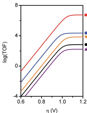
Fig. 5 Catalytic Tafel plots for **Fe-ortho-1-amide** (blue diamond), **Fe-ortho-2-amide** (red square), **Fe-para-1-amide** (purple upward triangle), **Fe-para-2-amide** (orange downward triangle), and **Fe-TPP** (black circle). Conditions: 0.1 M TBAPF<sub>6</sub> in DMF; 0.23 M  $\text{CO}_2$ ; 100 mM PhOH; scan rate is  $100 \text{ mV s}^{-1}$ .  $\text{TOF} = k_{\text{obs}}$  and was determined by FOWA.
