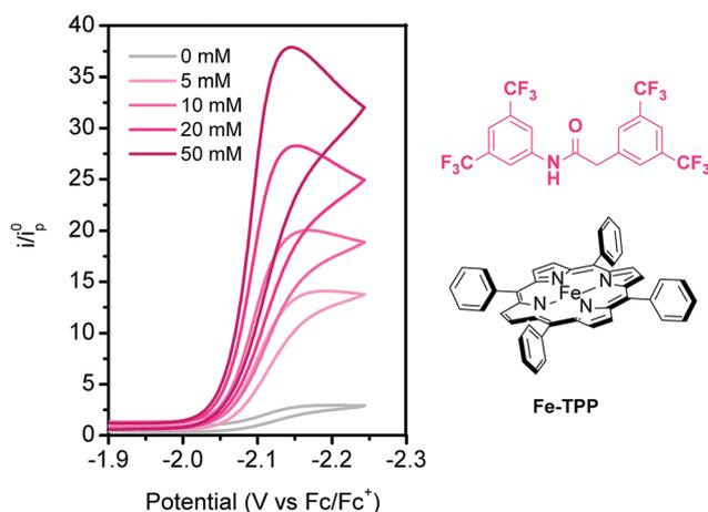
**Fig. 1** Titration of 3,5-bis(trifluoromethyl)phenyl]amide to **Fe-TPP** under CO<sub>2</sub> showing current increases with increasing concentrations of amide. Conditions: 0.1 M TBAPF<sub>6</sub> in DMF, 1 mM **Fe-TPP**.
