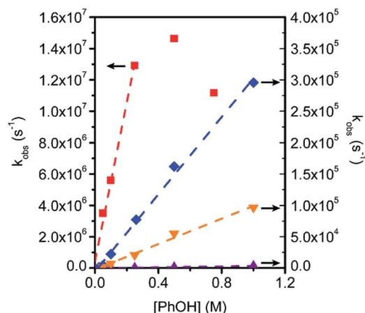
Fig. 4 Observed rate constants (s<sup>-1</sup>) for catalytic CO<sub>2</sub> reduction as a function of PhOH concentration for Fe-*ortho*-1-amide (blue diamonds), Fe-*ortho*-2-amide (red squares), Fe-*para*-1-amide (purple upward triangles), and Fe-*para*-2-amide (orange downward triangles). Conditions: 1 mM catalyst, 0.1 M TBAPF<sub>6</sub> in DMF, 0.23 M CO<sub>2</sub>; scan rate is 100 mV s<sup>-1</sup>.  $k_{\text{obs}}$  values were determined by FOWA.
