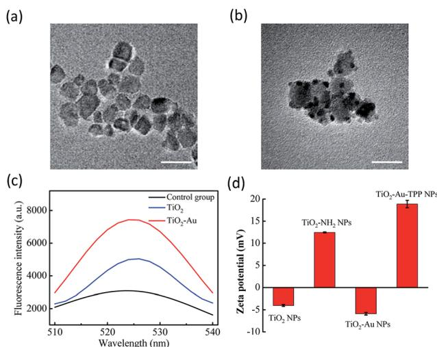
Fig. 1 Characterization of the nanoradiosensitizers. HRTEM images of the (a) TiO<sub>2</sub> NPs and (b) TiO<sub>2</sub>-Au NPs; the scale bars are 20 nm. (c) Fluorescence spectra of DBZTC (excitation = 490 nm, emission = 525 nm) after irradiation with X-rays. (d) Zeta potentials of each step of the modification: TiO<sub>2</sub> NPs; TiO<sub>2</sub>-NH<sub>2</sub> NPs; TiO<sub>2</sub>-Au NPs; and TiO<sub>2</sub>-Au-TPP NPs.
