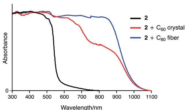
Fig. 9 Solid-state UV-vis-NIR absorption spectra of **2**, **2** + C<sub>60</sub> crystal, and **2** + C<sub>60</sub> fibre (spectra were normalized at 300 nm).
