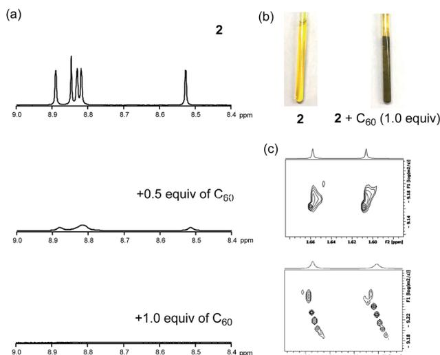
Fig. 5  $^1\text{H}$  NMR titration experiments of **2** in toluene- $d_8$ . (a)  $^1\text{H}$  NMR spectra of **2** (0.52 mM) with increasing amounts of  $C_{60}$ . (b) photographs of samples of **2** and **2** +  $C_{60}$ , and (c) DOSY measurements of **2** and **2** +  $C_{60}$ .
