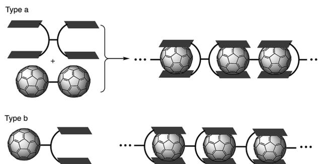
Fig. 1 Supramolecular polymerization of C<sub>60</sub> derivatives.
