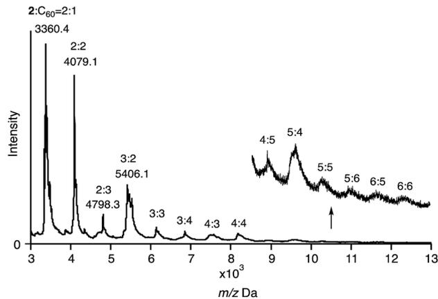
Fig. 8 MALDI-TOF MS spectrum of **2** with 1.0 equiv. of C<sub>60</sub> (matrix: *trans*-2-[3-(4-*tert*-butylphenyl)-2-methyl-2-propenylidene]malononitrile; DCTB).
