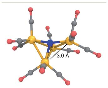
Fig. 5 Optimized structure of  $\mathbf{1}^{2-}$  at the BP86/6-31G\*-LANL2DZ level of theory, characterized by a "crooked butterfly" structure with a single elongated Fe–Fe distance of 3.0 Å. Fe, orange; C, grey; N, blue; O, red; H, white.
