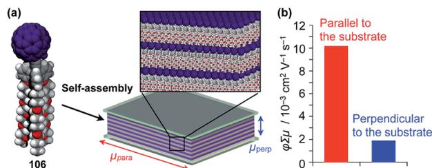
Fig. 17 (a) Schematic structure of an oriented 2D assembly of C<sub>60</sub> units achieved by a tripodal triptycene-based 2D supramolecular scaffold (**106**) and (b) its maximum transient conductivities ( $\phi \sum \mu$ ) sandwiched between quartz substrates along directions parallel (red) and perpendicular (blue) to the substrate as determined by flash-photolysis time-resolved microwave conductivity measurements.
