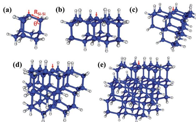
Fig. 1 The  $P_b$ -containing silicon clusters studied in this work. (a)  $Si_{10}H_{15}$  (sila-adamantane cluster), (b)  $Si_{22}H_{27}$ , (c)  $Si_{26}H_{31}$ , (d)  $Si_{47}H_{49}$  (1.3 nm SiNC), and (e)  $Si_{72}H_{63}$  (1.7 nm SiNC). One of the three symmetry-equivalent Si-Si bond lengths ( $R_{Si-Si}$ ) and bond angles ( $\theta$ ) discussed herein are indicated in red in (a). The red arrows indicate the positions of dangling bond defects.
