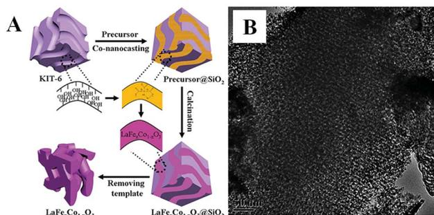
Fig. 1 (A) Synthesis process of the mesoporous LaFe<sub>x</sub>Co<sub>1-x</sub>O<sub>3</sub> perovskite oxides by co-nanocasting process using mesoporous KIT-6 as a hard template, (B) the as-prepared mesoporous LaFeO<sub>3</sub>. Reproduced with permission from ref. 34. Copyright© 2013, Royal Society of Chemistry.
