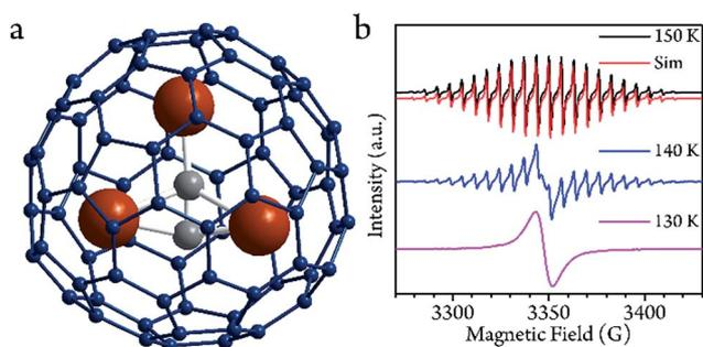
Fig. 1 (a) The optimized structure of the  $\text{Sc}_3\text{C}_2@\text{C}_{80}$  based on DFT calculations. (b) cw-EPR spectra from 130 to 150 K in  $\text{CS}_2$  solution. The spectrum at 150 K can be reproduced with the following parameters:  $g_{\text{iso}} = 2.00$  and  $A_{\text{iso}} = 18.10$  MHz. The simulation was performed by the EasySpin toolbox in the Matlab software.
