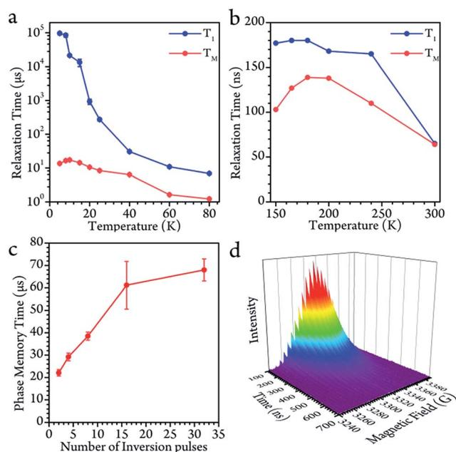
Fig. 3 (a and b) The longitudinal relaxation time ( $T_1$ ) and phase memory time ( $T_M$ ) in the low and high temperature regions. The spin echo signal is hard to record from 80 to 150 K. (c) The phase memory time enhanced by dynamic decoupling with various numbers of inversion pulses. (d) The spin echo decays as a function of the magnetic field.
