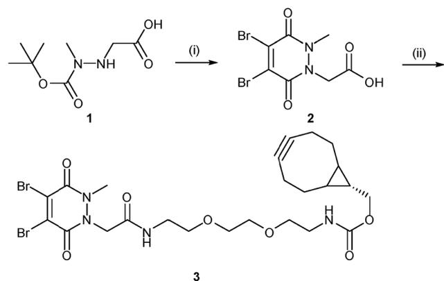
**Scheme 1** Synthesis of strained alkyne functionalised pyridazinedione **3**. Reagents and conditions: (i) dibromomaleic acid, AcOH, reflux, 24 h; (ii) PyBOP, DIPEA, CH<sub>2</sub>Cl<sub>2</sub>, 21 °C, 16 h.
