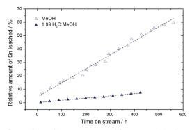
Fig. 5 Comparison of the percentage of Sn recovered in the reaction effluent relative to the initial tin content in the Sn-Beta catalyst during operation in methanol and 1:99 H<sub>2</sub>O:MeOH, as determined by ICP-MS.
