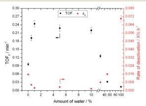
Fig. 2 Influence of solvent composition in terms of activity (TOF<sub>0</sub>) and rate of deactivation  $(k_d)$  during low temperature glucose-fructose isomerisation. Reaction conditions described in ESI† Table S1.
