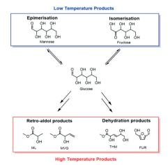
Scheme 1 General scheme demonstrating the products that can be obtained by the catalytic conversion of sugars with Sn-Beta at both low (<140 °C) and high (>140 °C) temperature.
