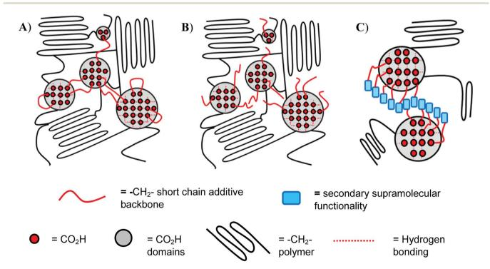
Fig. 1 Insertion of; (A) dicarboxylic acid additive (sebacic acid), (B) mono-carboxylic acid additive (dodecanoic acid), (C) creation of 'network within a network' via functionalised carboxylic acids additives to enable secondary supramolecular interactions into poly(ethylene-co-acrylic acid).
