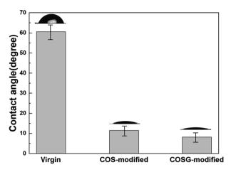
Fig. 8 Contact angles of the virgin, COS-modified and COSG-modified membranes.
