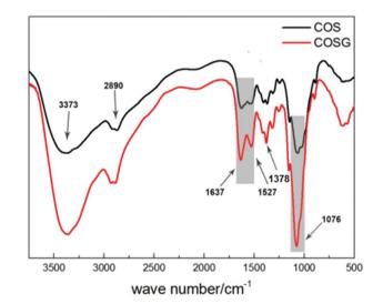
Fig. 4 FTIR spectra of COS and COSG
