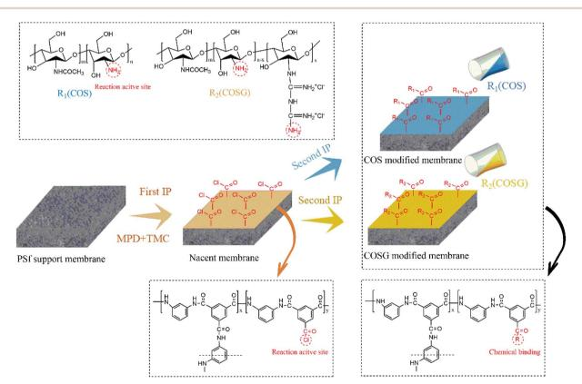
Fig. 3 Schematic diagram of the COS-modified and COSG-modified membrane fabrication process
