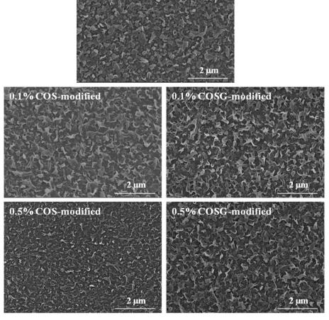
Fig. 6 SEM images of the virgin, COS-modified and COSG-modified membranes.
