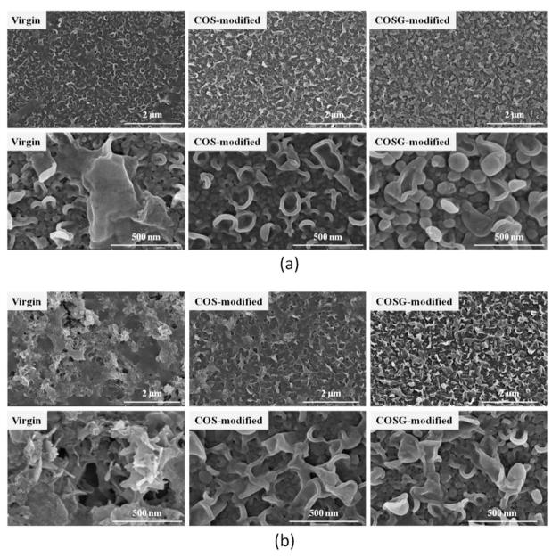
Fig. 10 SEM images of the RO membranes after BSA (a) and lysozyme (b) fouling (fouling condition: 2000 mg  $L^{-1}$  NaCl, 500 mg  $L^{-1}$  foulant,  $1.55~\text{MPa TMP}, 1.5~\text{L min}^{-1}, 25.0 \pm 0.1~\text{°C};$  rinsing condition: 2000 mg L $^{-1}$  NaCl, 0.62 MPa TMP, 4.0 L min $^{-1}$ ,  $25.0 \pm 0.1~\text{°C}).$
