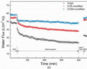
Fig. 9 The effect of BSA (a) and lysozyme (b) fouling on the water fluxes of the RO membranes (fouling condition: 2000 mg L $^{-1}$  NaCl, 500 mg L $^{-1}$  foulant, 1.55 MPa TMP, 1.5 L min $^{-1}$ , 25.0  $\pm$  0.1 °C; rinsing condition: 2000 mg L $^{-1}$  NaCl, 0.62 MPa TMP, 4.0 L min $^{-1}$ , 25.0  $\pm$  0.1 °C).
