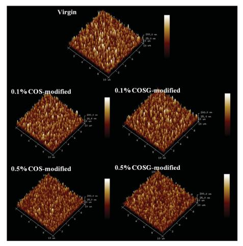
Fig. 7 AFM images of the virgin, COS-modified and COSG-modified membranes.
