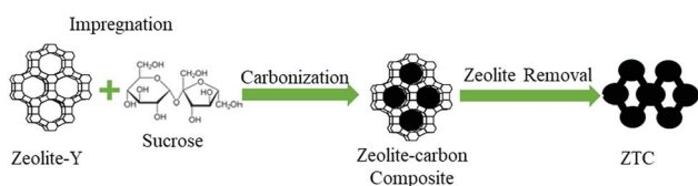
Fig. 1 Synthesis route of ZTC.
