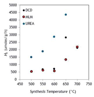
Fig. 7 H<sub>2</sub> evolution profiles obtained under simulated solar light using the g-C<sub>3</sub>N<sub>4</sub> samples as function of polymerization temperature and precursor type (RSDs < 5%, n = 3).
