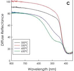
DRS spectra recorded on the q-C<sub>3</sub>N<sub>4</sub> samples obtained from (a) DCD, (b) MLM, (c) urea as function of synthesis temperature.
