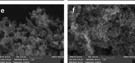
Fig. 3 SEM images collected on the g- $C_3N_4$  materials prepared from DCD (a, b), MLM (c, d) and urea (e, f) by thermal condensation at 500 °C (a, c, e), 700 °C (b, d) and 650 °C (f).
