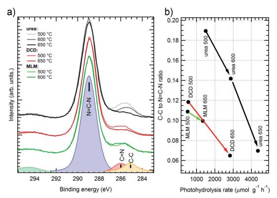
Fig. 6 (a) XPS spectra of C 1s peak of g-C<sub>3</sub>N<sub>4</sub> samples, obtained from urea (grey scale colors), DCD (red) and melamine (MLM, green); darker color corresponds to higher polymerization temperature. Peak fitting results for MM sample grown at 650 °C are shown on the bottom. (b) C-C/N=C-N peaks area ratio dependence on photocatalytic activity; arrows connect samples grown with the same precursor with the raising synthesis temperature.
