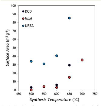
Fig. 8 Correlation between surface area and polymerization temperature for the g-C<sub>3</sub>N<sub>4</sub> catalysts.
