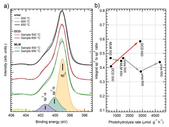
Fig. 5 (a) XPS spectra of N 1s peak on  $g-C_3N_4$  samples obtained from urea (grey scale colors), DCD (red) and melamine (MLM, green); darker color corresponds to higher polymerization temperature. Peak fitting results for MM sample grown at  $500 \,^{\circ}$ C are shown on the bottom. (b)  $\mathrm{sp}^2/\mathrm{sp}^3$  peaks area ratio dependence on photocatalytic activity; arrows connect samples grown from the same precursor with the raising synthesis temperature.
