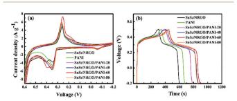
Fig. 4 CV profiles at 5 mV s<sup>-1</sup> (a) and galvanostatic charge–discharge curves at 1 A g<sup>-1</sup> (b) of  $SnS_2/NRGO$ , PANI, and  $SnS_2/NRGO/PANI$  with different amounts of PANI electrodes in 6 M KOH electrolyte.
