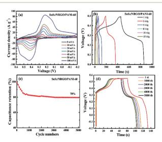
Fig. 6 Capacitive performances of  $SnS_2/NRGO/PANI-60$  based symmetric supercapacitor in 6 M KOH electrolyte: (a) CV profiles at different scan rates, (b) galvanostatic charge–discharge curves from 1 to 15 A  $g^{-1}$ , (c) cycling performance at 10 A  $g^{-1}$ , and (d) galvanostatic charge–discharge curves at  $1^{st}$ ,  $1000^{th}$ ,  $2000^{th}$ ,  $3000^{th}$ ,  $4000^{th}$  and  $5000^{th}$  cycles.
