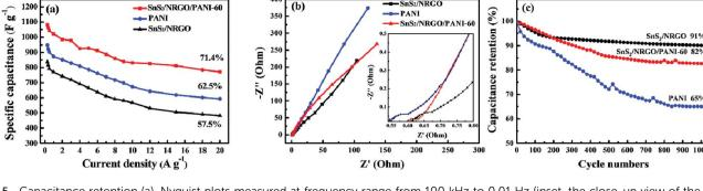
Fig. 5 Capacitance retention (a), Nyquist plots measured at frequency range from 100 kHz to 0.01 Hz (inset, the close-up view of the high-frequency region) (b), and cycling performances at 10 A  $\rm g^{-1}$  (c) of SnS<sub>2</sub>/NRGO, PANI, and SnS<sub>2</sub>/NRGO/PANI-60 hybrid electrodes in 6 M KOH electrolyte.
