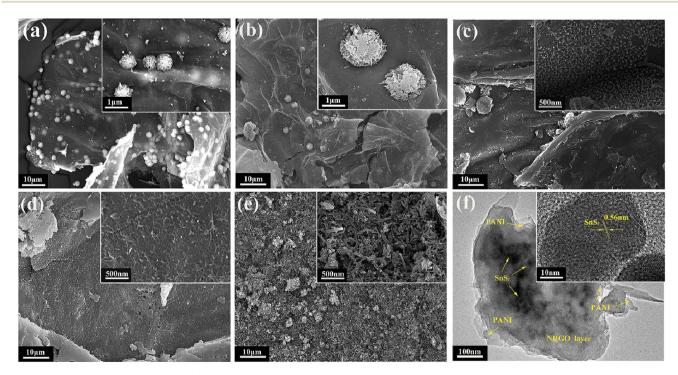
Fig. 2 SEM images of (a) SnS<sub>2</sub>/NRGO, (b) SnS<sub>2</sub>/NRGO/PANI-20, (c) SnS<sub>2</sub>/NRGO/PANI-40, (d) SnS<sub>2</sub>/NRGO/PANI-60, (e) SnS<sub>2</sub>/NRGO/PANI-80 and TEM images of (f) SnS<sub>2</sub>/NRGO/PANI-60.
