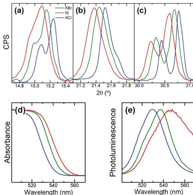
Fig. 2 XRD (a–c) and optical (d and e) characterization of powders prepared from  $\text{KI}$  (red),  $\text{KBr}$  (green), and  $\text{KCl}$  (blue). Shifts in diffractograms are consistent with the incorporation of the heteroanion ( $\text{I}$  or  $\text{Cl}$ ) in the perovskite structure. This translates into a smaller ( $\text{KI}$ ) or higher ( $\text{KCl}$ ) bandgap as observed in absorption (d) and photoluminescence (e).
