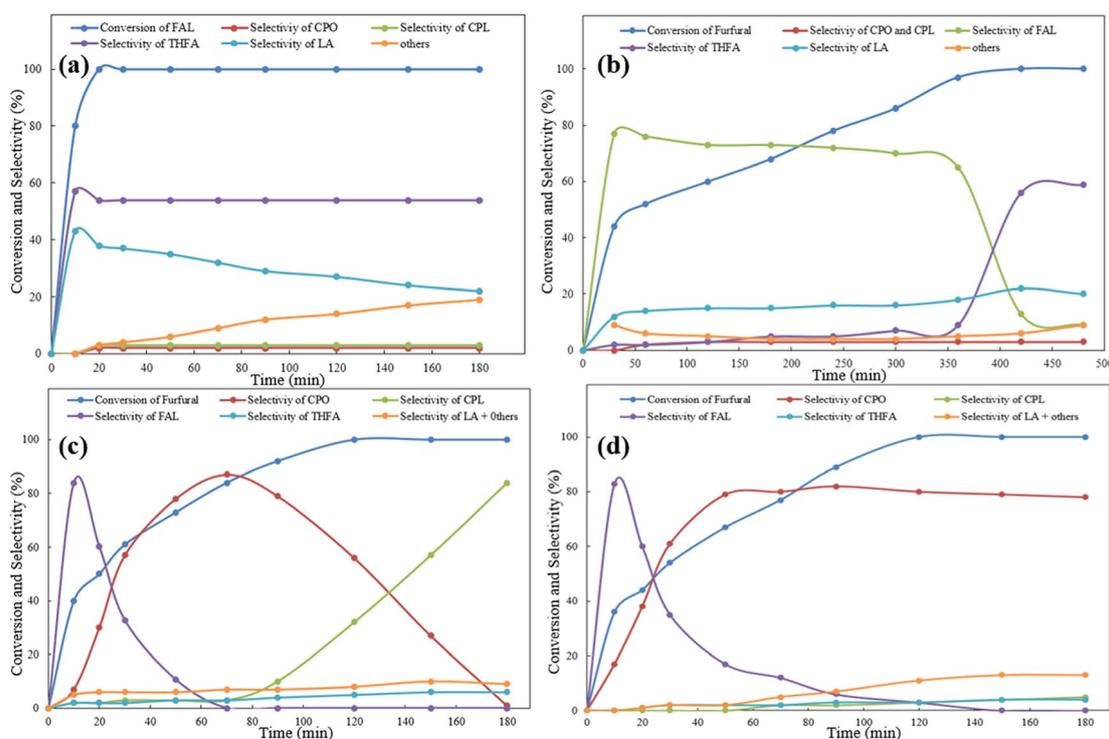
Fig. 2 Conversion and selectivity of different reaction conditions at different times. (a) Furfuryl alcohol (FAL) as the substrate, reacted at the temperature of 433 K, 4 MPa H<sub>2</sub>; (b) furfural as the substrate, reacted at the temperature of 393 K, 4 MPa H<sub>2</sub>; (c) furfural as the substrate, reacted at the temperature of 433 K, 4 MPa H<sub>2</sub>; and (d) furfural as the substrate, reacted at the temperature of 433 K, 2 MPa H<sub>2</sub>.
