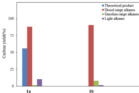
Fig. 5 Carbon yield of different alkanes from the HDO of different precursors over the Pd/C + H-beta system. The diesel range alkanes, gasoline range alkanes and light alkanes represent C<sub>9</sub>–C<sub>18</sub>, C<sub>5</sub>–C<sub>8</sub> and C<sub>1</sub>–C<sub>4</sub> alkanes, respectively.
