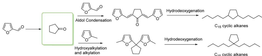
Scheme 3 Method for the synthesis of diesel range alkanes based on CPO from hemicellulose.
