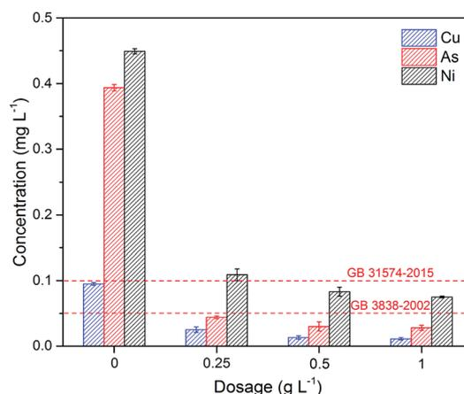
Fig. 6 The removal of As, Cu, and Ni by Fe<sub>3</sub>O<sub>4</sub>:S NPs in industrial wastewater. Experimental conditions: adsorbent dosage was 0.25–1 g L<sup>-1</sup>, contact time was 24 h, temperature was 30 °C (GB 31574-2015:<sup>47</sup> Emission standards of pollutants for secondary copper, aluminum, lead, and zinc industry; GB 3838-2002:<sup>48</sup> Environmental quality standards for surface water).
