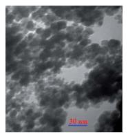
Fig. 4 TEM images of SO<sub>3</sub>H@imineZCMNPs.
