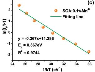
Fig. 7 (a) Temperature-dependent PL spectra of SGA:0.1%Mn<sup>4+</sup> phosphors under 353 nm excitation. (b) The normalized PL intensities of SGA:0.1%Mn<sup>4+</sup> phosphors at different temperature from 303 to 463 K. (c) The plot of  $\ln(I_0/I - 1)$  versus 1/kT.
