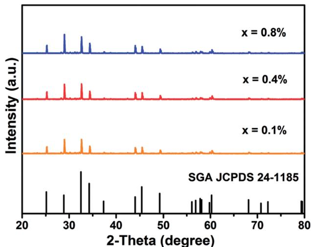
Fig. 1 XRD patterns of SGA:xMn<sup>4+</sup> (x = 0.1%, 0.4%, and 0.8%) phosphors and the standard profile of SGA (JCPDS no. 24-1185).
