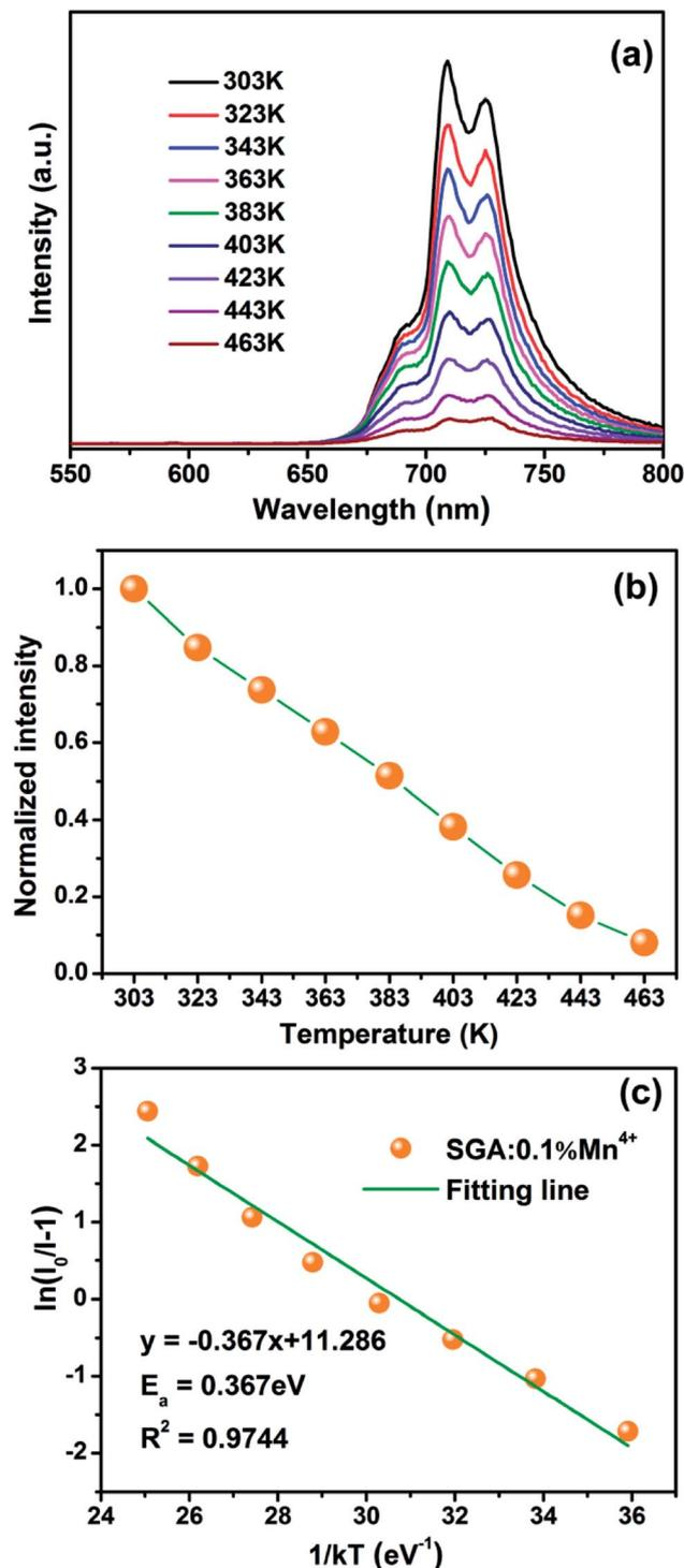
Fig. 7 (a) Temperature-dependent PL spectra of SGA:0.1%Mn<sup>4+</sup> phosphors under 353 nm excitation. (b) The normalized PL intensities of SGA:0.1%Mn<sup>4+</sup> phosphors at different temperature from 303 to 463 K. (c) The plot of  $\ln(I_0/I - 1)$  versus  $1/kT$ .
