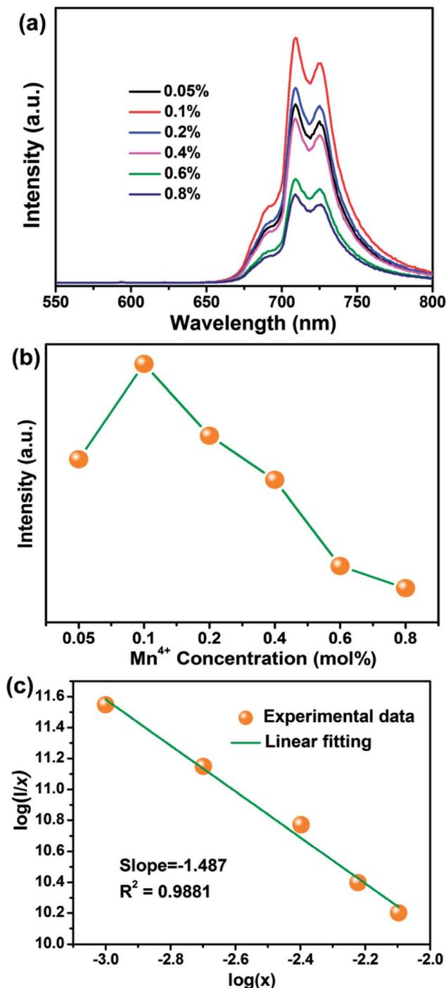
Fig. 4 (a) PL spectra of SGA: $x\text{Mn}^{4+}$  ( $x = 0.05\%$ ,  $0.1\%$ ,  $0.2\%$ ,  $0.4\%$ ,  $0.6\%$ , and  $0.8\%$ ) phosphors under 353 nm excitation. (b) PL intensity of SGA: $x\text{Mn}^{4+}$  as a function of  $\text{Mn}^{4+}$  doping concentrations. (c) Linear fitting of  $\log(I/x)$  versus  $\log(I/x)$  in SGA: $x\text{Mn}^{4+}$  phosphors excited at 353 nm.
