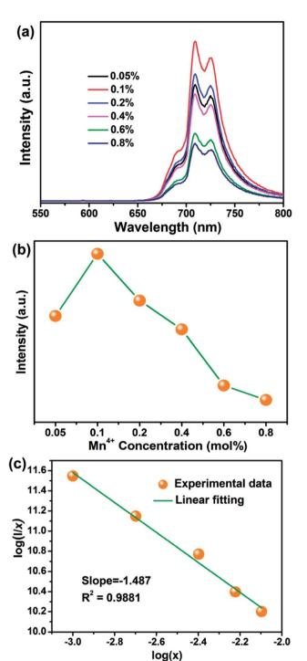
Fig. 4 (a) PL spectra of SGA:xMn<sup>4+</sup> (x = 0.05%, 0.1%, 0.2%, 0.4%, 0.6%, and 0.8%) phosphors under 353 nm excitation. (b) PL intensity of SGA:xMn<sup>4+</sup> as a function of Mn<sup>4+</sup> doping concentrations. (c) Linear fitting of log(x) versus log(x) in SGA:xMn<sup>4+</sup> phosphors excited at 353 nm.
