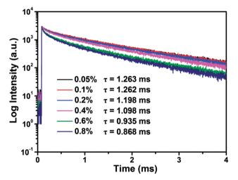
Fig. 6 Decay curves and calculated lifetimes of SGA:xMn $^{4+}$  (x=0.05%, 0.1%, 0.2%, 0.4%, 0.6%, and 0.8%) under 353 nm excitation and monitored at 709 nm.
