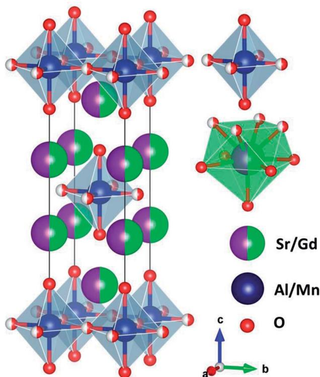
Fig. 2 Typical crystal structure of SGA and the Al<sup>3+</sup> and Sr<sup>2+</sup>/Gd<sup>3+</sup> sites are coordinated by six and nine oxygen atoms, respectively.
