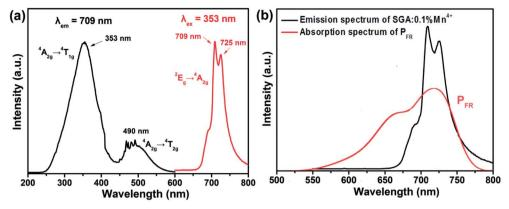
Fig. 3 (a) PLE and PL spectra of SGA:0.1%Mn<sup>4+</sup> phosphors. (b) PL spectrum of SGA:0.1%Mn<sup>4+</sup> phosphors and the absorption spectrum of
