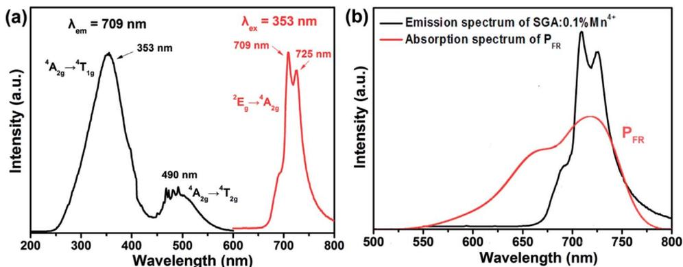
Fig. 3 (a) PLE and PL spectra of SGA:0.1%Mn<sup>4+</sup> phosphors. (b) PL spectrum of SGA:0.1%Mn<sup>4+</sup> phosphors and the absorption spectrum of phytochrome P<sub>FR</sub>.
