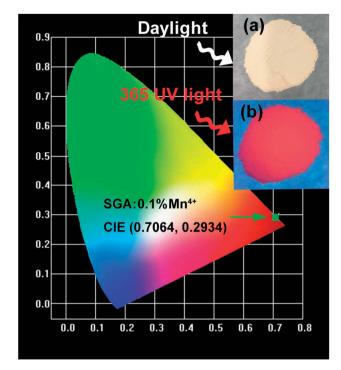
Fig. 5 CIE chromaticity coordinates of SGA:0.1%Mn<sup>4+</sup> phosphors under 353 nm excitation. The inset shows the digital photographs of SGA:0.1%Mn<sup>4+</sup> phosphors in daylight and under a 365 nm UV lamp.
