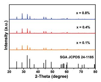
Fig. 1 XRD patterns of SGA:xMn<sup>4+</sup> (x = 0.1%, 0.4%, and 0.8%) phosphors and the standard profile of SGA (JCPDS no. 24-1185).
