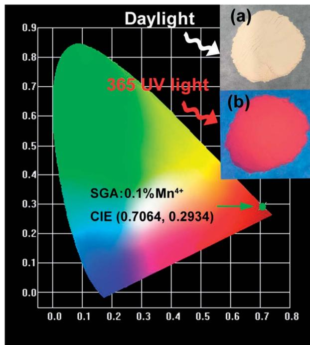
Fig. 5 CIE chromaticity coordinates of SGA: $0.1\%\text{Mn}^{4+}$  phosphors under 353 nm excitation. The inset shows the digital photographs of SGA: $0.1\%\text{Mn}^{4+}$  phosphors in daylight and under a 365 nm UV lamp.
