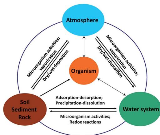
Fig. 1 The geochemical cycles of arsenic in Nature.
