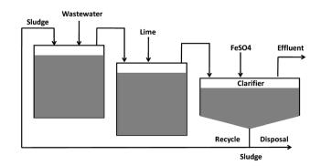
Fig. 2 A typical method for the removal of high concentrations of arsenic from water.
