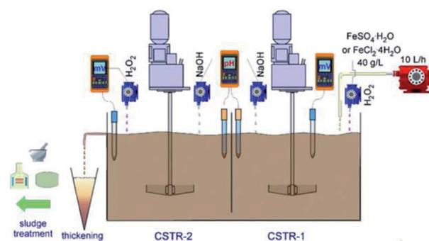
Fig. 3 Scheme of the laboratory iron oxy-hydroxides' production.<sup>52</sup>
