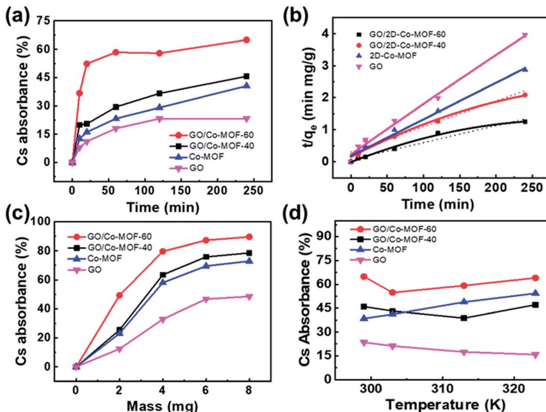
Fig. 3 (a) Effects of contact time on the adsorption of  $\text{Cs}^+$  on GO/Co-MOF membranes; (b) the time-dependent sorption pseudo-second-order kinetic plots (solid lines) of  $\text{Cs}^+$  removal on GO, Co-MOF, GO/2D-Co-MOF-40 and GO/2D-Co-MOF-60. (c) Effect of adsorbent dosage on the adsorption of  $\text{Cs}^+$  on GO/Co-MOF membranes. (d) Effects of temperature on the adsorption of  $\text{Cs}^+$  on GO/Co-MOF membranes.
