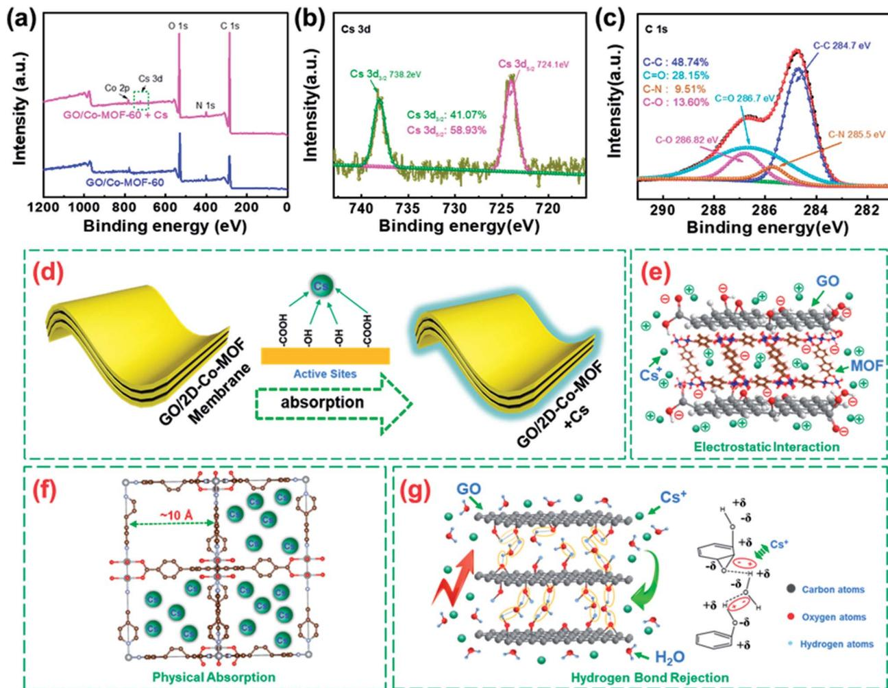
Fig. 4 (a) The XPS spectra of GO/Co-MOF before and after  $\text{Cs}^+$  sorption; (b) the Cs 3d XPS spectrum of GO/Co-MOF after  $\text{Cs}^+$  sorption; (c) the C 1s XPS spectrum of GO/Co-MOF after  $\text{Cs}^+$  sorption; (d) sorption mechanism of  $\text{Cs}^+$  on GO/Co-MOF samples; (e) schematic of mechanisms of sorption reaction in GO/Co-MOF composite membranes; (f) Schematic of mechanisms of sorption reaction in Co-MOF; (g) Schematic of mechanisms of sorption reaction in GO membranes.
