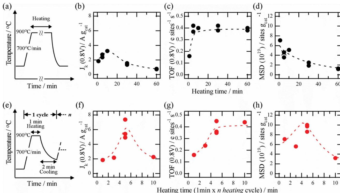
Fig. 3 (a) Profile of continuous heating process. Time evolution of (b)  $J_k$ , (c) TOF, and (d) MSD of catalyst prepared by a process. (e) Profile of short and repeated heating process. Time evolution of (f)  $J_k$ , (g) TOF, and (h) MSD of catalyst prepared by (e) process.
