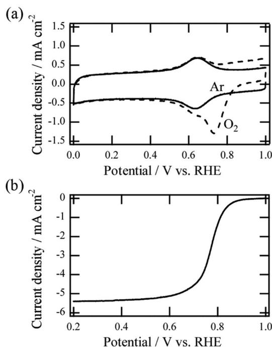
Fig. 2 (a) Representative CV curves of Fe–N–C/VACNT catalysts in O<sub>2</sub>-saturated (dotted line) and Ar-saturated (solid line) 0.5 M H<sub>2</sub>SO<sub>4</sub> solutions. (b) RDE curves of Fe–N–C/VACNT catalyst at 1600 rpm in the O<sub>2</sub> saturated acid media.
