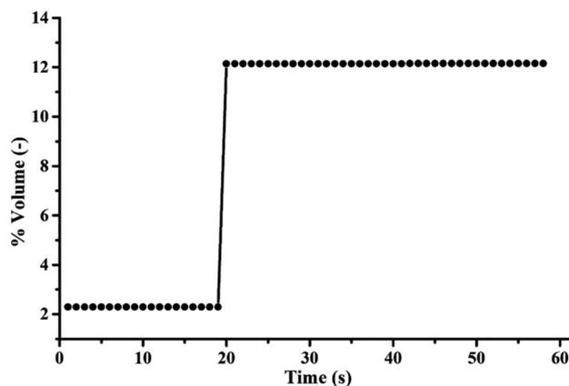
Fig. 8 Breakthrough curve of the optimum operating condition (sorption temperature of 60 °C, superficial gas velocity of 0.22 m s<sup>-1</sup>, sorbent packing of 5 g).
