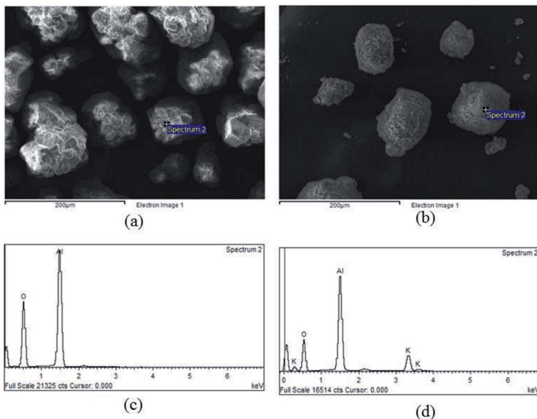
Fig. 3 Textural properties of a sorbent before adsorbing CO<sub>2</sub>, (a) SEM image of  $\gamma$ -Al<sub>2</sub>O<sub>3</sub>, (b) SEM image of sorbent, (c) EDX pattern of  $\gamma$ -Al<sub>2</sub>O<sub>3</sub>, (d) EDX pattern of sorbent.
