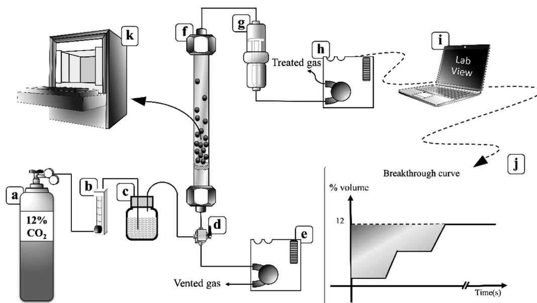
Fig. 2 Fluidization sorption system.<sup>40</sup>
