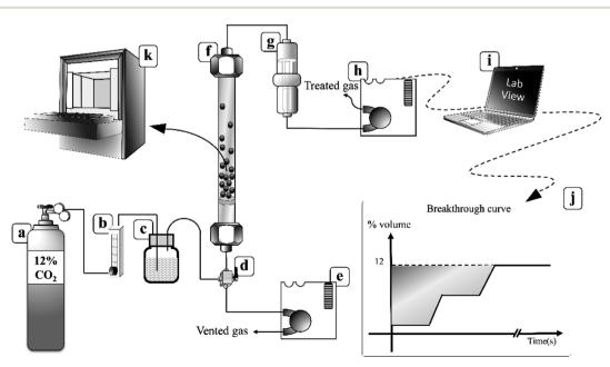
Fig. 2 Fluidization sorption system. 40
