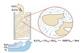
Fig. 1 CO<sub>2</sub> sorption in turbulent fluidized bed (TFB) riser.
