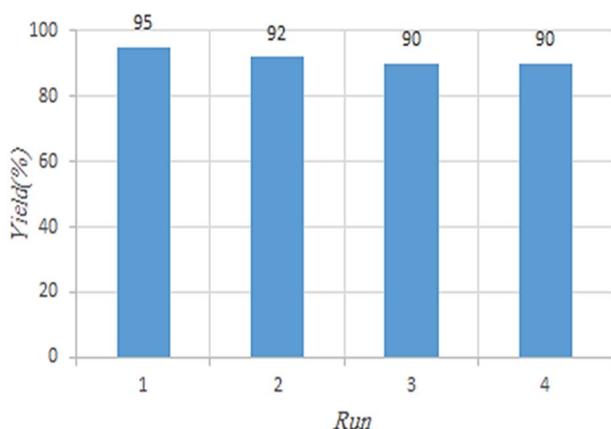
Fig. 6 Recyclability of C(MIM-PTA)<sub>4</sub> in the Mannich reaction.
