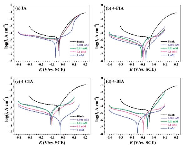
Fig. 3 Potentiodynamic polarization curves recorded for copper in  $0.5 \,\mathrm{M}\,\mathrm{H}_2\mathrm{SO}_4$  solution containing different concentrations of the investigated inhibitors at 298 K, (a) IA, (b) 4-FIA (c) 4-CIA, (d) 4-BIA.
