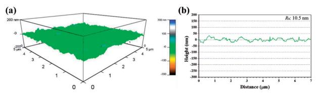
Fig. 10 (a) 3D AFM graph and (b) height profile of copper specimen after immersion in 0.5 M H<sub>2</sub>SO<sub>4</sub> solution in the presence of 1 mM 4-CIA for 8 h at 298 K.
