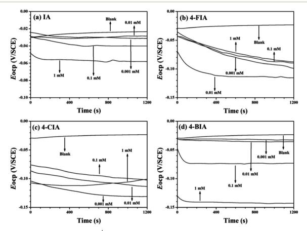
Fig. 2 OCP-time curves for copper in  $0.5 \text{ mol L}^{-1} \text{ H}_2\text{SO}_4$  solution containing different concentrations of the investigated inhibitors at 298 K, (a) IA, (b) 4-FIA (c) 4-CIA, (d) 4-BIA.
