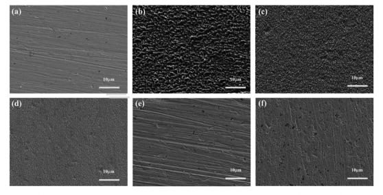
Fig. 7 FE-SEM images of (a) freshly polished copper specimen and the specimens immersed in  $0.5 \,\mathrm{M}\,\mathrm{H}_2\mathrm{SO}_4$  solution (b) without and with  $1 \,\mathrm{mM}$ (c) IA, (d) 4-FIA, (e) 4-CIA, (f) 4-BIA for 32 h at 298 K.
