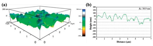
Fig. 9 (a) 3D AFM graph and (b) height profile of copper specimen after immersion in  $0.5 \,\mathrm{M}\,\mathrm{H}_2\mathrm{SO}_4$  solution in the presence of 1 mM IA for 8 h at 298 K.
