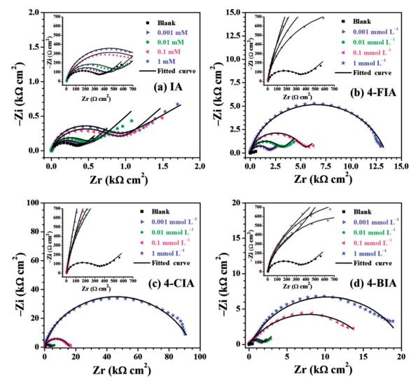
Fig. 4 Nyquist plots for the copper electrode in 0.5 M H<sub>2</sub>SO<sub>4</sub> solution without and with different concentrations of (a) IA, (b) 4-FIA (c) 4-CIA, (d) 4-BIA at 298 K.
