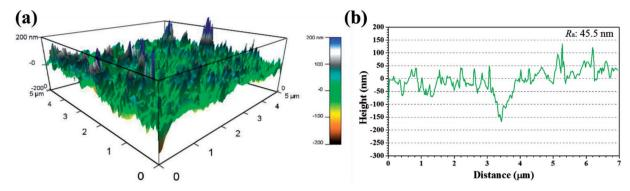
Fig. 8 (a) 3D AFM graph and (b) height profile of copper specimen after immersion in 0.5 M H<sub>2</sub>SO<sub>4</sub> solution without inhibitors for 8 h at 298 K.
