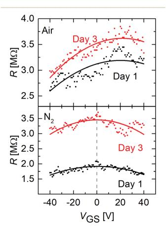
Fig. 5 Resistance of FGS with a C/O ratio of x = 26 versus gate voltage for different days under air (top) and nitrogen (bottom) atmosphere.
