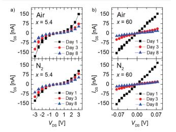
Fig. 2  $I_{\rm DS}/V_{\rm DS}$  characteristics of selected single FGS transistor devices for C/O ratios (a) x=5.4 and (b) x=60 under air (top) and N<sub>2</sub> (bottom) atmosphere at different days. The gate of the device was left unconnected (floating gate).
