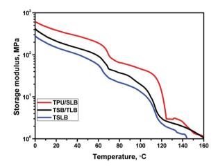
The storage modulus curves of the specimens.
