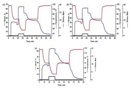
The triple-shape memory cycles with T<sub>s</sub>'s of 70 and 125 °C of the (a) TSLB, (b) TSB/TLB, and (c) TPU/SLB specimens.
