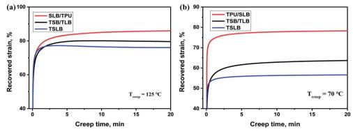
Evolution of recovered strain of the specimens during the creeping progresses at (a) 125 °C and (b) 70 °C.
