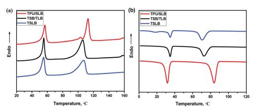
Fig. 4 DSC (a) heating and (b) cooling curves of the specimens.
