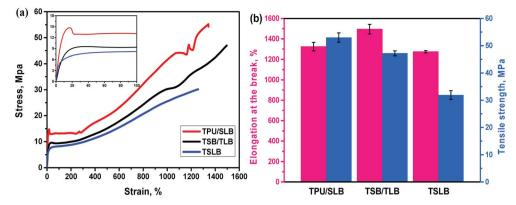
Fig. 10 (a) Stress-strain curves of the specimens (the inset shows the enlarged part of the curves); (b) comparison of tensile strength and elongation at break among the specimens.
