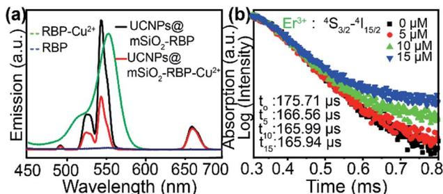
Fig. 1 (a) The absorbance spectrum of RBP-Cu<sup>2+</sup> and RBP and the emission spectrum of UCNPs@mSiO<sub>2</sub>-RBP and UCNPs@mSiO<sub>2</sub>-RBP-Cu<sup>2+</sup> in the ethanol–water solution. (b) Er<sup>3+</sup> decay curves recorded for UCNPs@mSiO<sub>2</sub>-RBP with different concentrations of Cu<sup>2+</sup> from 0 to 15 μM in the ethanol–water solution.
