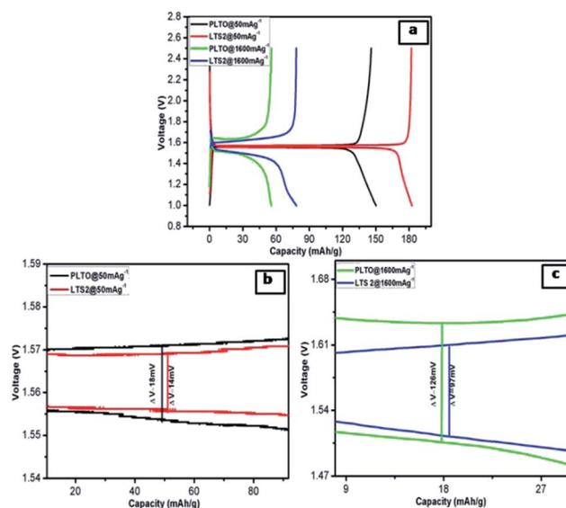
Fig. 10 (a) Comparison of the initial discharge-charge profiles of PLTO and LTS2 at 50 and 1600 mA g<sup>-1</sup> and (b) 50 mA g<sup>-1</sup> (c) 1600 mA g<sup>-1</sup>.
