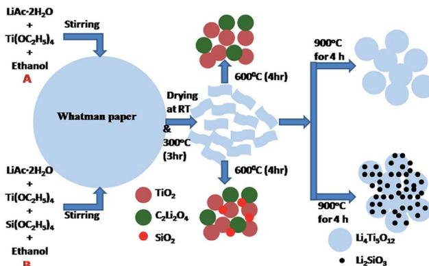
Fig. 1 Schematic diagram of the formation mechanism process of the LTO and surface modified LTO.
