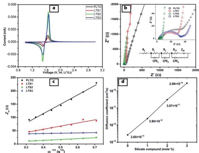
Fig. 8 (a) Cyclic voltammograms of all LTO samples (PLTO, LTS1, LTS2 and LTS3) electrode at a scan rate of  $0.2 \text{ mV s}^{-1}$ . (b) Electrochemical impedance spectrum and inset is enlarged spectra in the high-medium frequency region and equivalent circuit model. (c) The relationship between  $Z_{re}$  and  $\omega^{-1/2}$ . (d) The relationship between  $\text{Li}^+$  diffusion coefficient with mole% of silicate compound.
