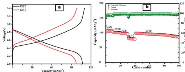
Fig. 11 (a) Galvanostatic charge–discharge voltage profiles of a LiCoO<sub>2</sub>/LTS2 full cell at varied current densities within a voltage of 2–3.4 V; (b) the rate performance for LiCoO<sub>2</sub>/LTS2 full cell.
