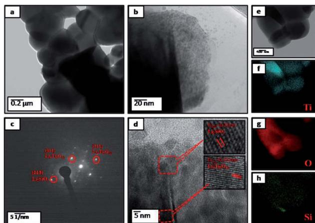
Fig. 5 FETEM images of pristine silicate modified  $\text{Li}_4\text{Ti}_5\text{O}_{12}$  (LTS2) (a and b) at different magnifications; (c) corresponding SAED patterns; (d) HRTEM of the individual  $\text{Li}_4\text{Ti}_5\text{O}_{12}$  (e) STEM image of  $\text{Li}_4\text{Ti}_5\text{O}_{12}$  and EDS mappings: colour map of (f) Ti, (g) O and (h) Si.
