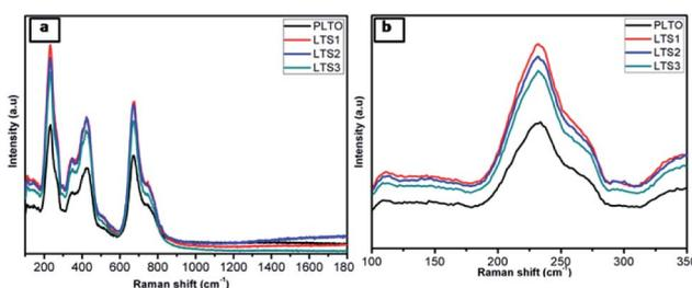
Fig. 6 Raman spectra of (a) all  $\text{Li}_4\text{Ti}_5\text{O}_{12}$  (PLTO, LTS1, LTS2 and LTS3) samples (b) compares the magnified Raman signature.
