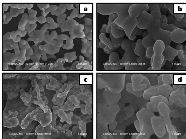
Fig. 3 FESEM images of (a and b) pristine  $\text{Li}_4\text{Ti}_5\text{O}_{12}$  (PLTO) and (c and d) the silicate modified  $\text{Li}_4\text{Ti}_5\text{O}_{12}$  (LTS2) at low and high magnifications.
