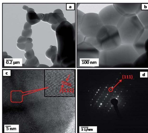
Fig. 4 FETEM images of pristine  $\text{Li}_4\text{Ti}_5\text{O}_{12}$  (PLTO) (a and b) at different magnifications; (c) FETEM of the individual  $\text{Li}_4\text{Ti}_5\text{O}_{12}$  at high resolution; (d) corresponding SAED patterns.
