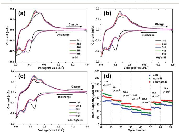
Fig. 4 Cyclic voltammograms of the first five cycles of (a) pure a-Si, (b) Ag/a-Si, and (c) a-Si/Ag/a-Si thin film electrodes in the voltage window (vs. Li/Li<sup>+</sup>) of 0.01–1.5 V at a scan rate of 0.1 mV s<sup>-1</sup>; (d) the rate capabilities of the pure a-Si, Aq/a-Si, and a-Si/Aq/a-Si thin film electrodes.
