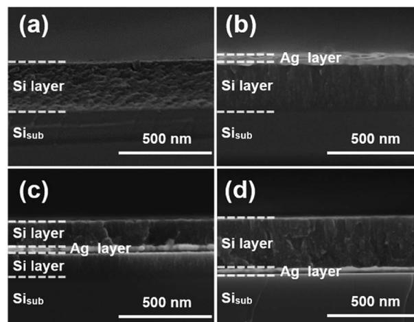
Fig. 1 Cross-sectional SEM images of the Si–Ag film with different positions of the Ag thin layer: (a) Si (280 nm)/Si<sub>sub</sub>; (b) Ag (30 nm)/Si (280 nm)/Si<sub>sub</sub>; (c) Si (140 nm)/Ag (30 nm)/Si (140 nm)/Si<sub>sub</sub>; (d) Si (280 nm)/Ag (30 nm)/Si<sub>sub</sub>. “Si<sub>sub</sub>” stands for silicon substrate.
