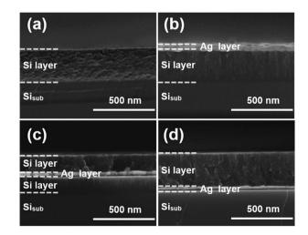
Fig. 1 Cross-sectional SEM images of the Si–Ag film with different positions of the Ag thin layer: (a) Si (280 nm)/Si $_{\rm sub}$ ; (b) Ag (30 nm)/Si (280 nm)/Si $_{\rm sub}$ ; (c) Si (140 nm)/Ag (30 nm)/Si (140 nm)/Si $_{\rm sub}$ , (d) Si (280 nm)/Ag (30 nm)/Si $_{\rm sub}$ . "Si $_{\rm sub}$ " stands for silicon substrate.
