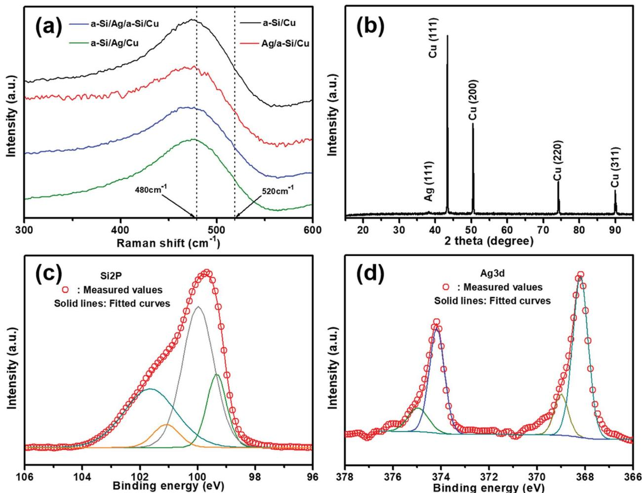
Fig. 2 (a) Raman spectra of the pristine a-Si (280 nm)/Cu (9  $\mu\text{m}$ ), Ag (30 nm)/a-Si (280 nm)/Cu (9  $\mu\text{m}$ ), a-Si (140 nm)/Ag (30 nm)/a-Si (140 nm)/Cu (9  $\mu\text{m}$ ) and a-Si (280 nm)/Ag (30 nm)/Cu (9  $\mu\text{m}$ ) electrodes; (b) XRD pattern of a-Si/Ag/a-Si/Cu multilayer electrode; XPS spectra: (c) Si 2p spectra and (d) Ag 3d spectra of a-Si/Ag/a-Si multilayer film deposited by the sputtering method. The top silicon layer is removed by Ar ion etching.
