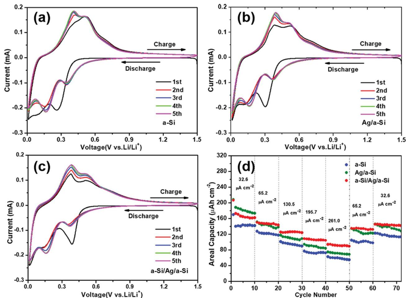
Fig. 4 Cyclic voltammograms of the first five cycles of (a) pure a-Si, (b) Ag/a-Si, and (c) a-Si/Ag/a-Si thin film electrodes in the voltage window (vs. Li/Li<sup>+</sup>) of 0.01–1.5 V at a scan rate of  $0.1 \text{ mV s}^{-1}$ ; (d) the rate capabilities of the pure a-Si, Ag/a-Si, and a-Si/Ag/a-Si thin film electrodes.
