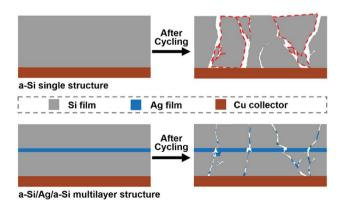
Fig. 9 Schematic illustration of the mechanism of an a-Si/Ag/a-Si electrode for improving the electrochemical performance. The areas marked by red dashed lines represent the inactive silicon materials after cycling. After cleaning, the inactive silicon materials are removed and the surface of the copper foil will be exposed
