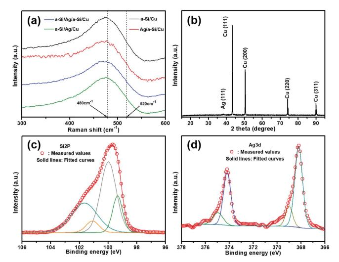
Fig. 2 (a) Raman spectra of the pristine a-Si (280 nm)/Cu (9  $\mu$ m), Ag (30 nm)/a-Si (280 nm)/Cu (9  $\mu$ m), a-Si (140 nm)/Ag (30 nm)/a-Si (140 nm)/Cu (9  $\mu$ m) and a-Si (280 nm)/Ag (30 nm)/Cu (9  $\mu$ m) electrodes; (b) XRD pattern of a-Si/Ag/a-Si/Cu multilayer electrode; XPS spectra: (c) Si 2p spectra and (d) Ag 3d spectra of a-Si/Ag/a-Si multilayer film deposited by the sputtering method. The top silicon layer is removed by Ar ion etching.
