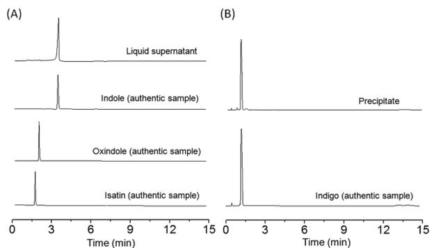
**Fig. 5** HPLC analysis of (A) the components extracted from the liquid supernatant of reaction mixture and monitored at 280 nm, and (B) the precipitate monitored at 250 nm catalyzed by F43Y Mb. HPLC traces of authentic samples of oxindole, isatin and indigo were shown for comparison.
