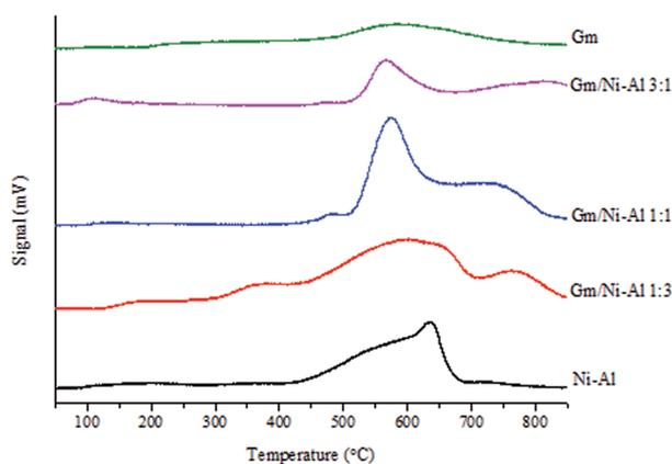
Fig. 5 TPD-NH<sub>3</sub> profiles for synthesized catalysts.
