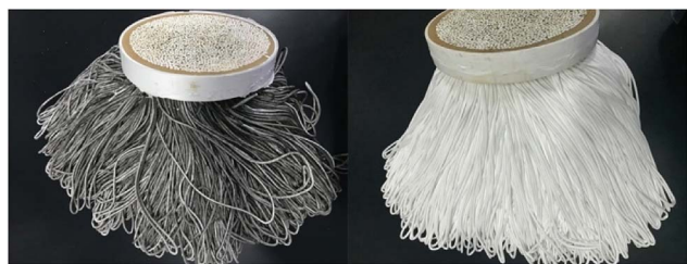
Fig. 13 PTFE hollow fiber membrane module after air filtration and the new module.
