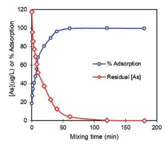
Fig. 3 Kinetics of adsorption of arsenic onto nZIF-8. Initial concentration =  $117\,\mu g\,L^{-1}$ . 80 mg nZIF-8, 800 mL solution, sampling volume = 0.1 mL, replicates = 3, mixing temperature = 25 °C, mixing rate = 130 rpm.
