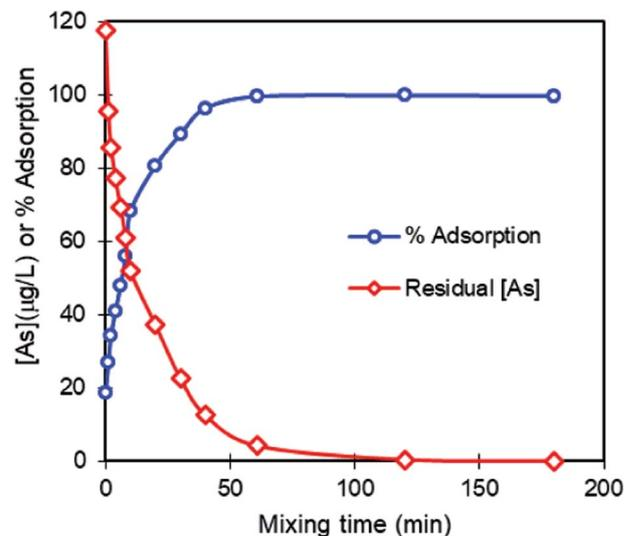
Fig. 3 Kinetics of adsorption of arsenic onto nZIF-8. Initial concentration =  $117 \mu\text{g L}^{-1}$ . 80 mg nZIF-8, 800 mL solution, sampling volume = 0.1 mL, replicates = 3, mixing temperature =  $25^\circ\text{C}$ , mixing rate = 130 rpm.
