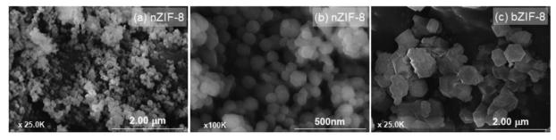
Fig. 2 SEM images showing the finer and homogeneously distributed (a and b) nZIF-8 particles in comparison with those of (c) bZIF-8.
