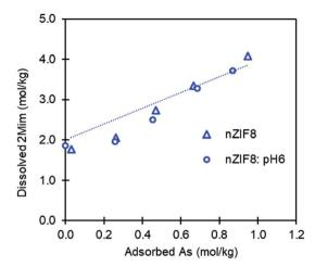
Fig. 6 Dissolved 2Mim (TOC-based) showing the mole to mole exchange of  ${\rm HAsO_4}^{2-}$  with 2Mim.
