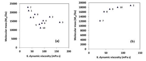
Fig. 1 Correlation between the mass-average molecular mass ( $M_{\rm w}$ ) for Novozym 435-catalyzed ROP-produced polyester and the dynamic viscosity (30 °C) of the IL medium (the number next to each symbol indicates the IL shown in Table 1) for (a) poly( $\iota$ -lactide) and (b) poly( $\iota$ -caprolactone) synthesis.
