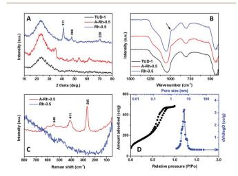
Fig. 1 (A) XRD patterns of the neat TUD-1, as synthetized Rh-TUD-1 (A-Rh-0.5) and Rh-0.5 sample. (B) The corresponding FTIR spectra. (C) Raman spectra of A-Rh-0.5 compared to Rh-0.5 sample. (D) The  $\rm N_2$  sorption isotherms of Rh-0.5 sample together with the pore size distribution.
