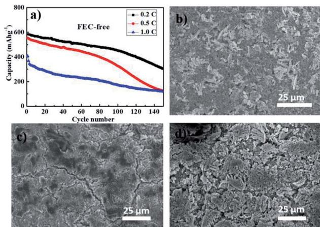
Fig. 5 (a) Cycling performances of the composite FeS<sub>2</sub> cathode in a FEC-free electrolyte at different C rates in 0.7–2.4 V range. SEM images of the dendritic FeS<sub>2</sub> composite cathode (b) before the cycling test, (c) after 150 cycles at 0.2C in FEC-free electrolyte and (d) after 150 cycles at 0.2C in 10 wt% FEC-containing electrolyte.
