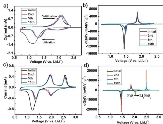
Fig. 3 Electrochemical properties of the dendritic  $\text{FeS}_2$  composite cathode at different cycle. CV at a scan rate of  $0.2 \text{ mV s}^{-1}$  over (a) 0.7–2.4 V and (c) 0.7–3.0 V; differential capacity versus voltage over (b) 0.7–2.4 V and (d) 0.7–3.0 V at 0.2C.
