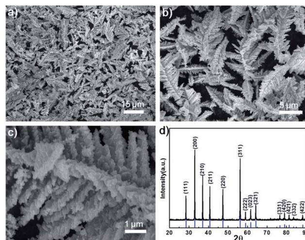
Fig. 1 (a) Low, (b) intermediate and (c) high magnification SEM images of dendritic nanostructured FeS<sub>2</sub>; (d) XRD pattern of as-synthesized FeS<sub>2</sub> with JCPDS card 65-7643 included below the spectra.
