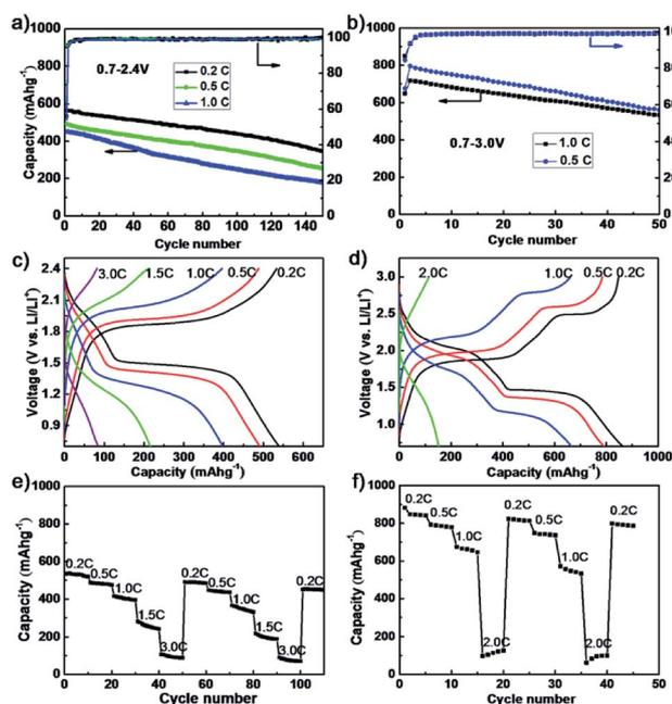
Fig. 2 Cycling stability of the dendritic  $\text{FeS}_2$  composite electrodes (a) between 0.7–2.4 V at 0.2C, 0.5C and 1C, and (b) between 0.7–3.0 V at 0.5C and 1.0C; voltage–capacity curves in (c) 0.7–2.4 V and (d) 0.7–3.0 V range; and consecutive rate capability (e) from 0.2C to 3C over 0.7–2.4 V and (f) from 0.2C to 2C over 0.7–3.0 V.
