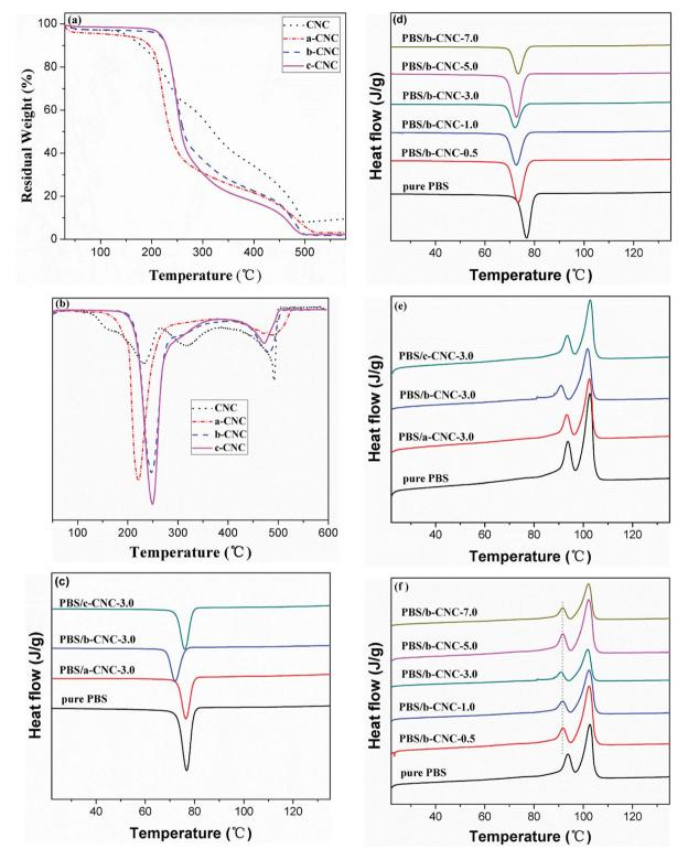
Fig. 7 (a) TGA and (b) DTG curves of CNC, a-CNC, b-CNC, and c-CNC; (c and d) DSC cooling and (e and f) the second heating scans of pure PBS and PBS/modified CNC composites.
