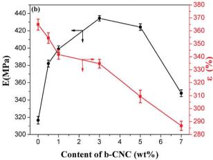
Fig. 10 Effect of (a) the a-CNC, b-CNC, and c-CNC content on the tensile modulus of the PBS composites and (b) b-CNC content on the tensile modulus and elongation at fracture of the PBS/b-CNC composites.
