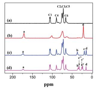
Fig. 5 Solid-state  $^{13}$ C NMR analysis of (a) CNC, (b) a-CNC, (c) b-CNC, and (d) c-CNC.
