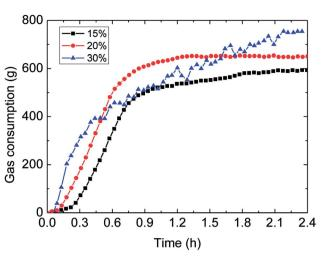
Fig. 8 The influence of the water-cut on gas consumption (1.0 m s $^{-1}$  flow rate, control temperature 1 °C, 6 MPa).
