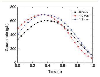
Fig. 12 The influence of flow rate on the growth rate (control temperature -1 °C, 6 MPa, 15% water-cut).
