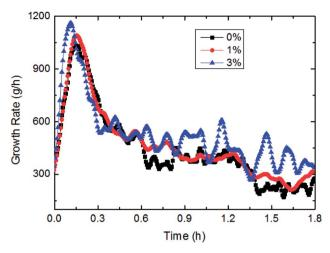
Fig. 16 The influence of the AA concentration on the growth rate  $(1.2 \text{ m s}^{-1} \text{ flow rate, } 6.5 \text{ MPa, } 30\% \text{ water-cut, control temperature } -1 ^{\circ}\text{C}).$
