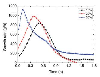
Fig. 9 The influence of the water-cut on the growth rate (1.0 m s $^{-1}$  flow rate, control temperature 1 °C, 6 MPa).
