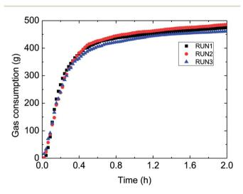
Fig. 4 Gas consumption during three reproduced formation experiments in the flow-loop (15% water-cut, 5 MPa, 1.0 m s $^{-1}$  flow rate).
