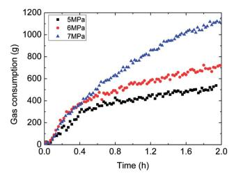
Fig. 6 The influence of the initial experimental pressure on the gas consumption (1.0 m s $^{-1}$  flow rate, control temperature 1 °C, 30% water-cut).
