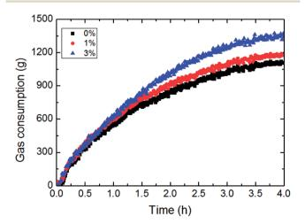
Fig. 15 The influence of the AA concentration on the gas consumption (1.2 m s<sup>-1</sup> flow rate, 6.5 MPa, 30% water-cut, control temperature -1 °C).
