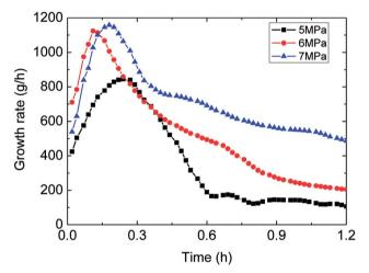
Fig. 7 The trend of growth rate against with time (1.0 m s $^{-1}$  flow rate, control temperature 1 °C, 30% water-cut).
