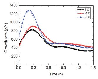
Fig. 14 The influence of the temperature set on the growth rate  $(0.6 \text{ m s}^{-1} \text{ flow rate, } 6 \text{ MPa, } 30\% \text{ water-cut)}$
