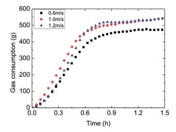
Fig. 11 The influence of flow rate on the gas consumption (control temperature  $-1\,^{\circ}$ C, 6 MPa, 15% water-cut).
