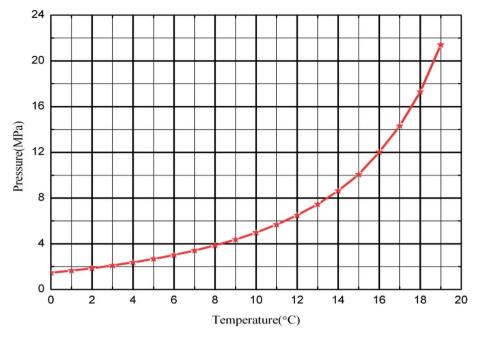
Fig. 2 Hydrate formation curve of test natural gas
