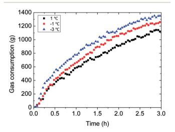
Fig. 13 The influence of the temperature set on the gas consumption (0.6 m s<sup>-1</sup> flow rate, 6 MPa, 30% water-cut)
