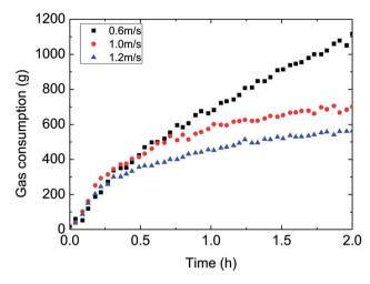
Fig. 10 The influence of flow rate on the gas consumption (control temperature -1 °C, 6 MPa, 30% water-cut).
