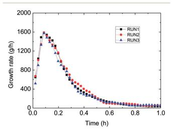
Fig. 5 Growth rate (gas consumption) during three reproduced formation experiments in the flow-loop (15% water-cut, 5 MPa,  $1.0~{\rm m~s^{-1}}$  flow rate).
