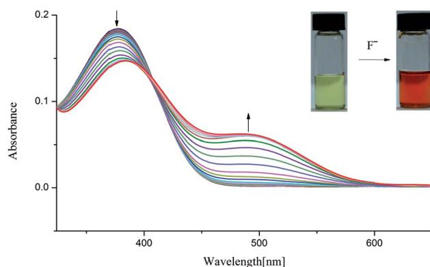
Fig. 3 Changes in UV-Vis spectra for L2 with addition of TBAF in DMSO solution ( $[L2] = 1.0 \times 10^{-5}$  M).
