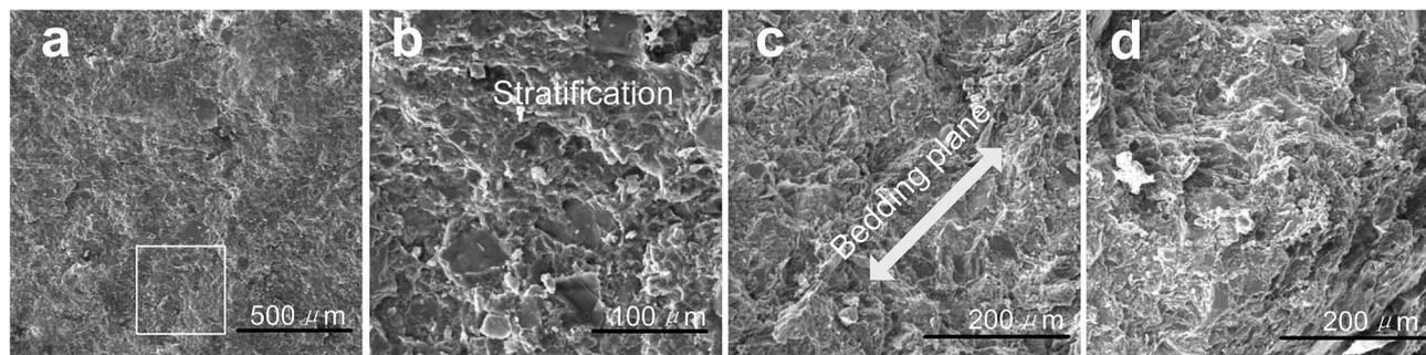
Fig. 12 SEM images of fracture surface of shale samples; (a) and (b) are the surface of transverse fractures with the magnification of  $\times 100$  and  $\times 500$ ; (c) and (d) are the surface of longitudinal fractures with the magnification of  $\times 300$  and  $\times 300$ .
