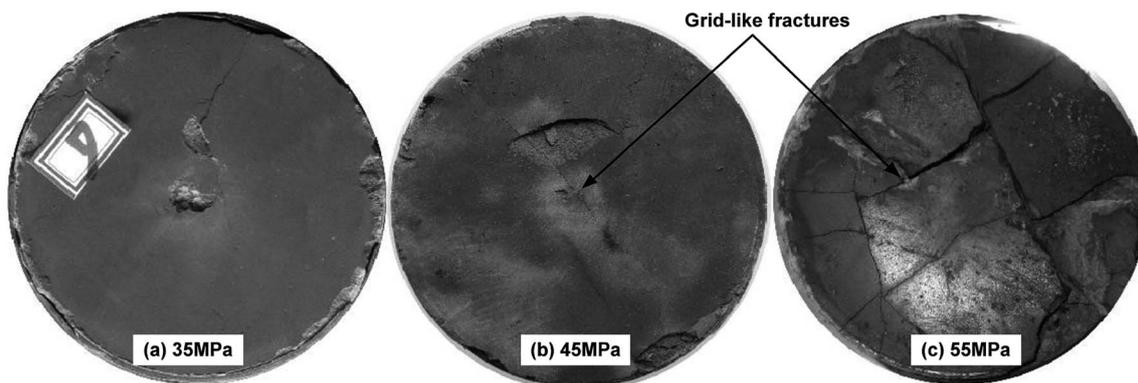
Fig. 4 Pictures of head faces of shale-cores impacted by SC-CO<sub>2</sub> jet with different pump pressures.
