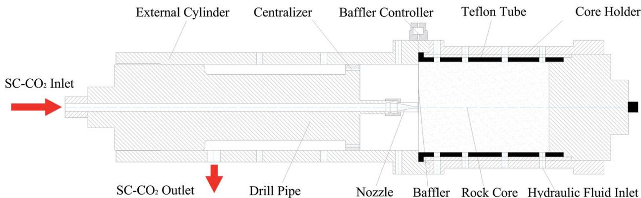
Fig. 2 Schematic diagram of the SC-CO<sub>2</sub> jet impacting rock apparatus.
