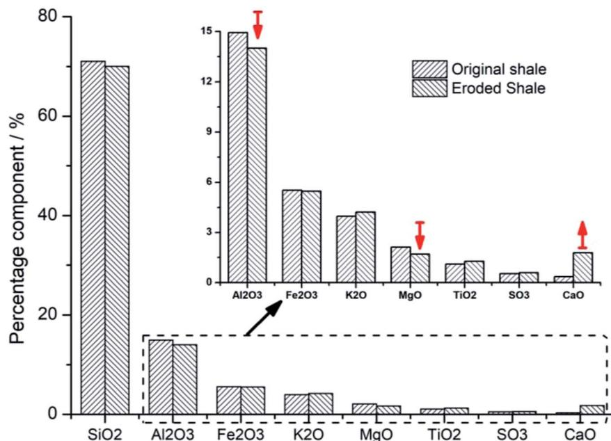
Fig. 10 Contrast of components in shale samples before and after the SC-CO<sub>2</sub> jet impacting.
